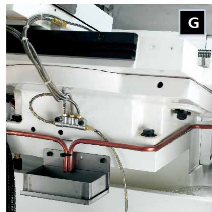
Lubrication Oil Recycle Lubrication oil for all slideways flow return through brass tubes to oil collecting tanks. This not only helps to maintain a clean working area, but also meets ISO-14000 environmental protection requirements.
